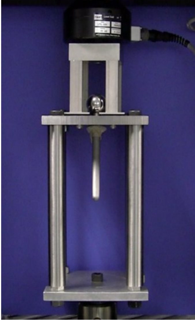
Figure 1-7. Custom test frame for head dissociation testing, Drexel University
